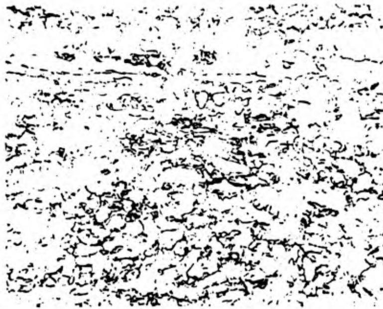
Figure 29. Longitudinal Section of Sheet 5895 After Rolling at 1121 C. Bright Field Illumination at 250 X
