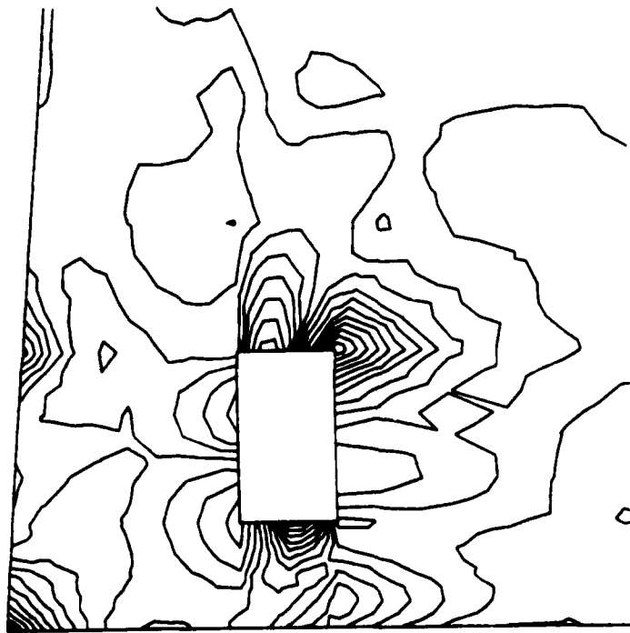
Figure B34. Window plot of nonannotated, Y-direction principal stress contours, fine grid, P-level 5
