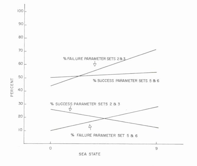
FIGURE 3-10. EVENT SUCCESS AND FAILURE AS A FUNCTION OF SEA STATE.
