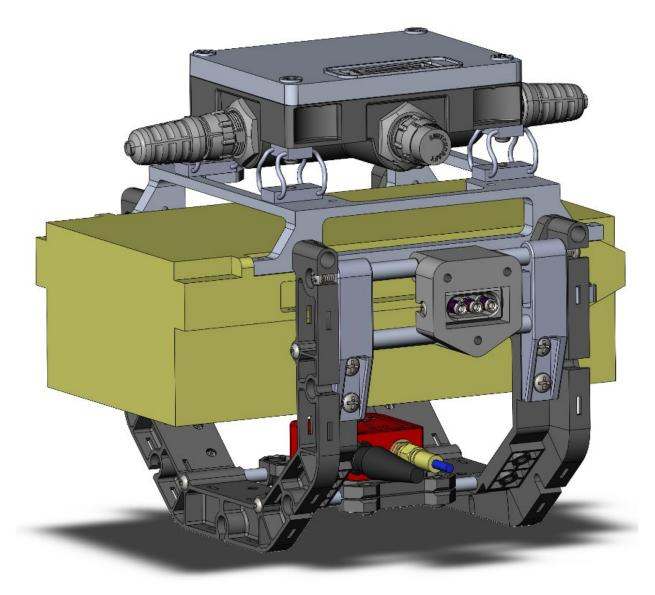
Figure F-6. SkyRaider Primary Mount with 2U Payload and INS
