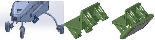
Figure C-13. TigerShark Main Payload Bay 45° Antenna Mount
