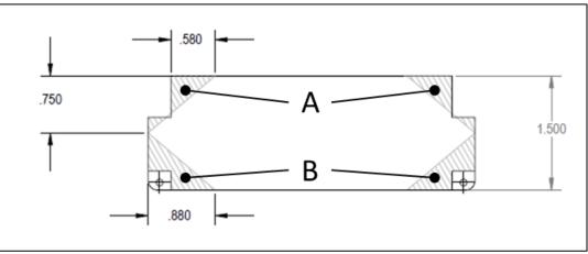
Figure 3-8. Connector Keep Out Zones
