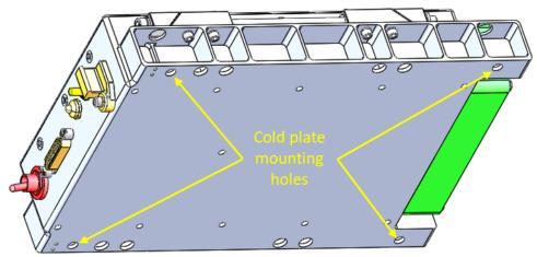
Figure 3-11. Payload Configured for Cold Plate Mounting
