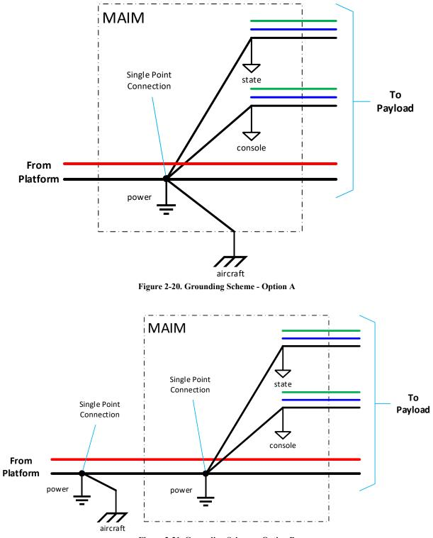
Figure 2-21. Grounding Scheme - Option B
