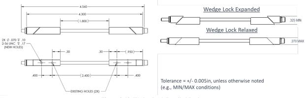
Figure 3-10. Wedge Lock Detailed Design
