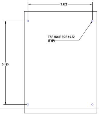
Figure 2-11. MP-compliant Plate Primary Mount Interface
