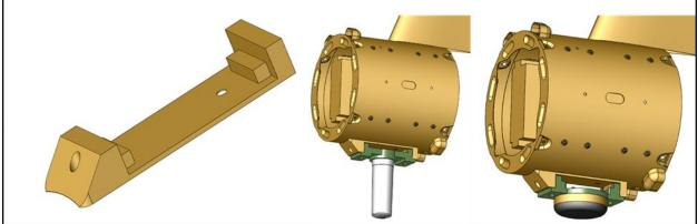
Figure B-11. Sled Antenna Mounts on the Aft Slice Primary Mount
