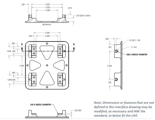
Figure 2-17. MP-compliant 4-pt Mount Interface
