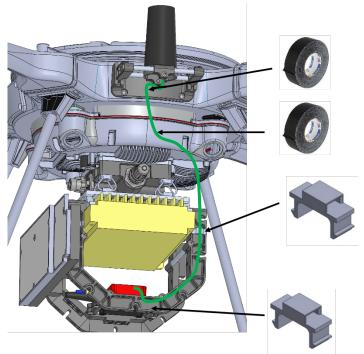
Figure F-21. SkyRaider GPS Antenna Cable Routing
