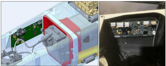
Figure E-5. MAIM Installed on Stalker
