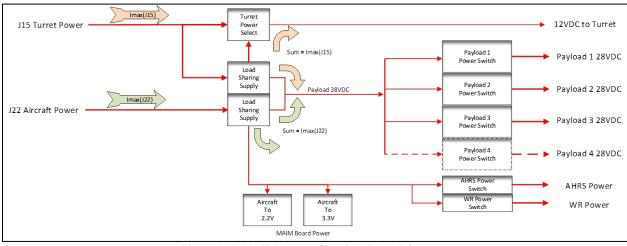
Figure B-5. MAIM Power Circuitry Block Diagram
