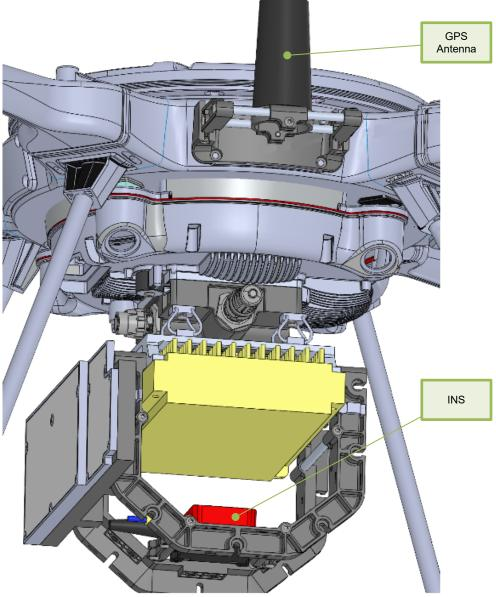
Figure F-10. SkyRaider INS and GPS Antenna
