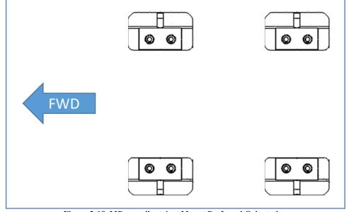
Figure 2-18. MP-compliant 4-pt Mount Preferred Orientation
