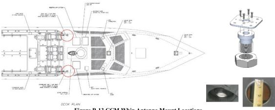
Figure B-13 CCM Whip Antenna Mount Locations
