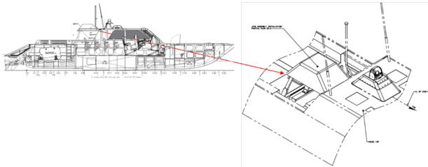
Figure B-6 CCM Primary Antenna Mount
