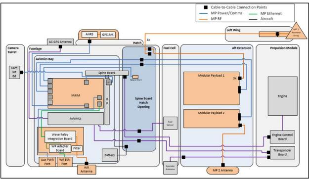
Figure B-13. MP Cables and Routing for Scan Eagle
