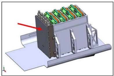
Figure D-6. MAIM Installed on Jump-20 MP Payload Tray
