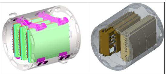
Figure B-7. Scan Eagle Primary Mount Aft Slice with Payloads
