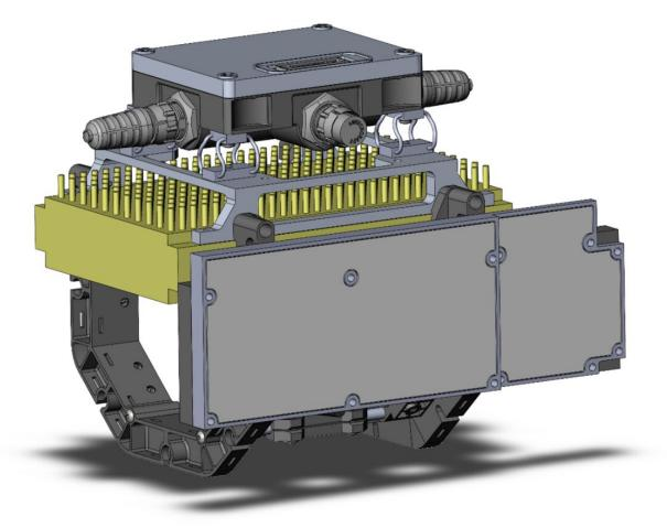
Figure F-9. SkyRaider Primary Mount with Payload Installed with Heatsink
