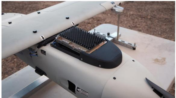
Figure E-6. Stalker Primary Mount with 1U Payload
