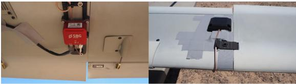
Figure E-11. Stalker INS and GPS Antenna
