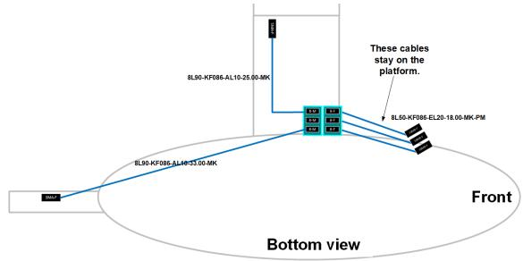
Figure E-23. Stalker RF Cables – Two Antenna Configuration
