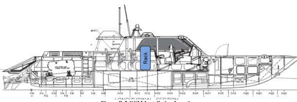
Figure B-2 CCM Installation Location
