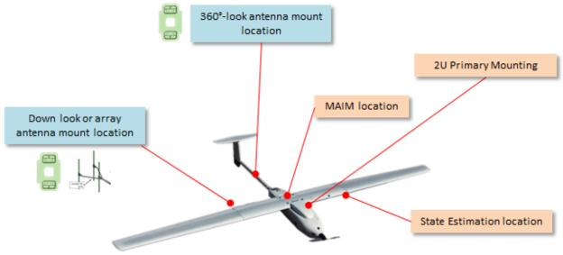
Figure E-1. Architectural Layout for MP-Stalker
