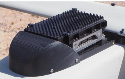
Figure E-10 Stalker Primary Mount – Payload Installation (3 of 3)
