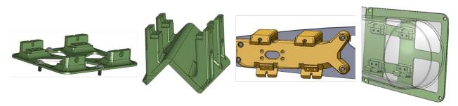
Figure 2-16. Example MP-compliant 4-pt Mounts
