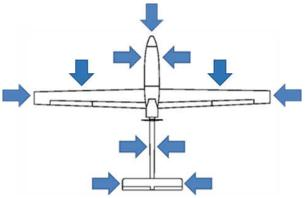
Figure 2-12. Possible MP Antenna Placements
