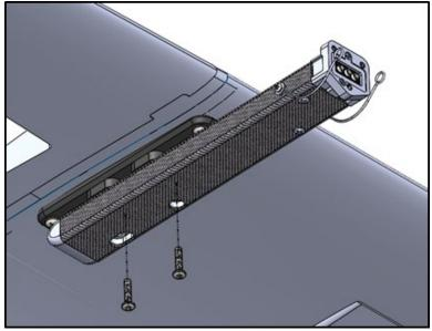
Figure E-12. Stalker Array (Strut) Mount
