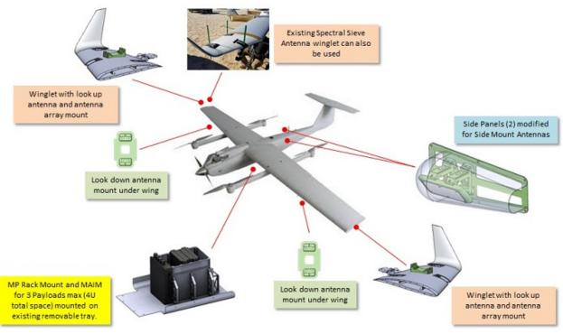
Figure D-1. Architectural Layout for MP-Jump-20
