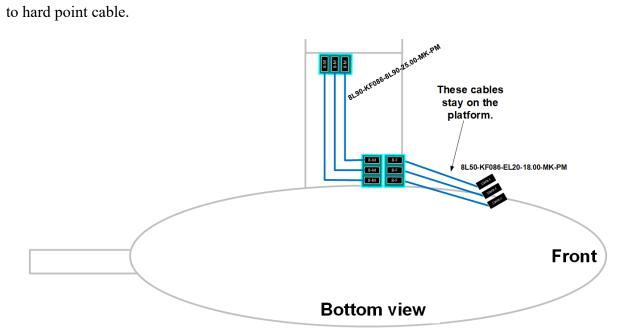
Figure E-21. Stalker RF Cables – Array Configuration
