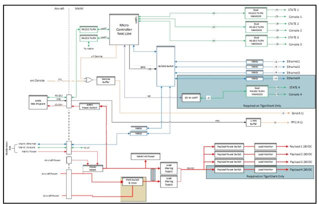
Figure 2-2. Example MAIM Block Diagram
