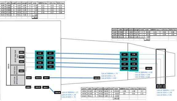
Figure D-24. Jump-20 Right RF Cables
