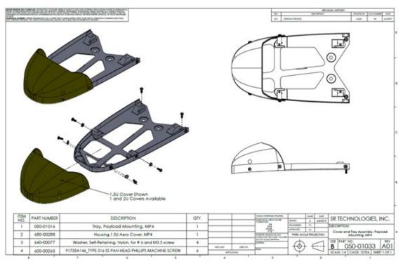
Figure E-7. Stalker Primary Mount Assembly Drawing
