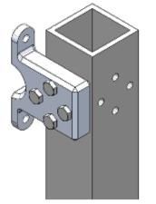
Figure 1-9 B-kit Antenna Mount Example
