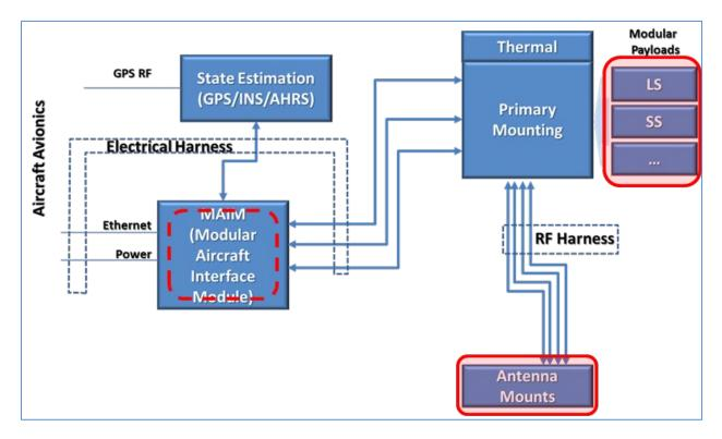
Figure 2-1. MP Block Diagram
