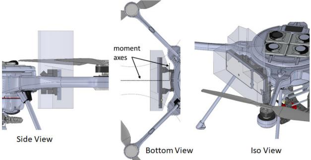
Figure F-13. SkyRaider Universal 2-pt Mount Allowable Antenna Volume
