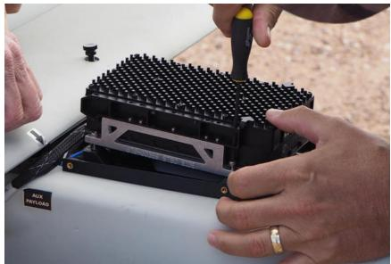
Figure E-9. Stalker Primary Mount – Payload Installation (2 of 3)
