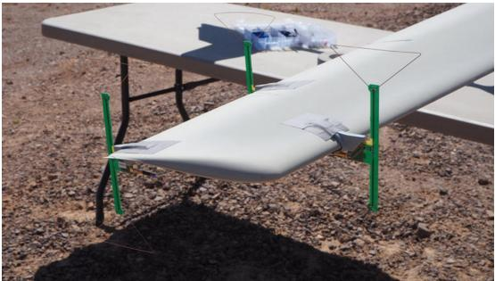
Figure E-26. Non-compliant SURFR3B Antenna Array
