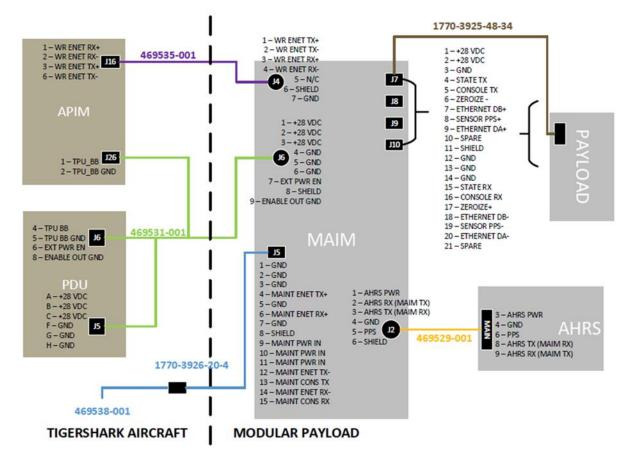
Figure C-16. TigerShark MAIM Cabling Schematic
