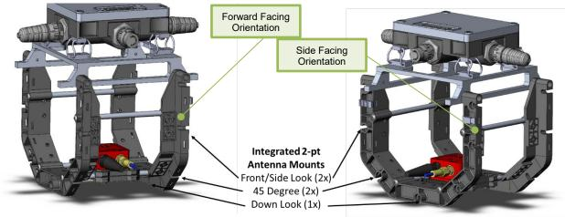
Figure F-14. Mounting Locations on the Antenna Mounting Frame
