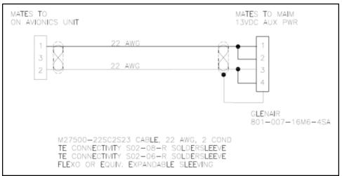
Figure D-19. MAIM Secondary Power Cable Pinout
