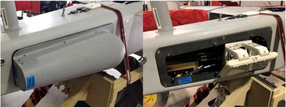
Figure D-16. Jump-20 Side Hatch Antenna Mount – With Radome (left), Without Radome (right)
