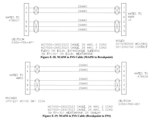
As shown in Figure E-20, the MAIM-INS cables run from the top of the MAIM through an exhaust port on the left side of the fuselage, to and along the bottom of the wing to the INS, mounted to the hard point at the left edge of the center wing. The inline breakpoint is located at the wing root. In total, the MAIM-INS cables are 50-inches long and weigh 52g.
