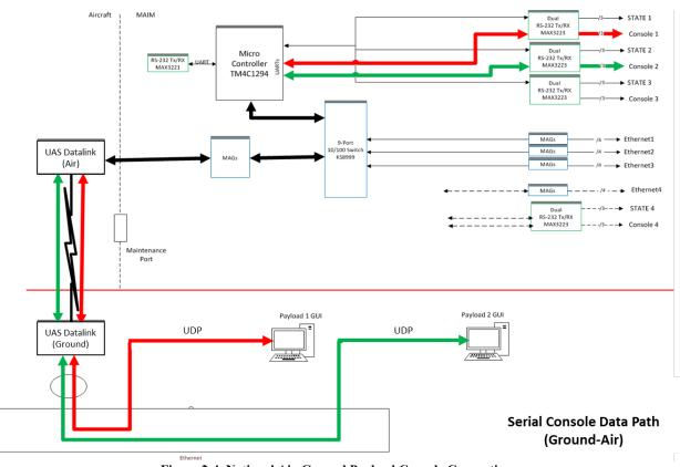
Figure 2-4. Notional Air-Ground Payload Console Connections
