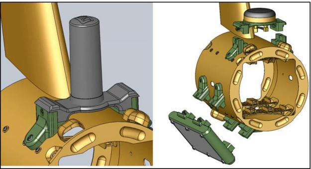
Figure B-10. Feet Antenna Mounts on the Aft Slice Primary Mount
