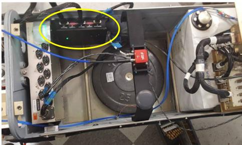
Figure C-6. MAIM Installed in TigerShark Payload Bay
