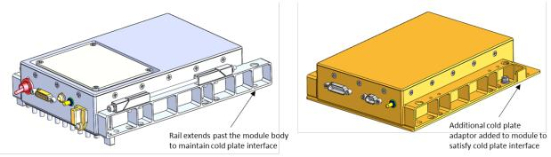
Figure 3-7. Example Reduced Length Modules
