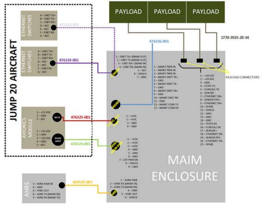
Figure D-17. Jump-20 MAIM Cabling Schematic
