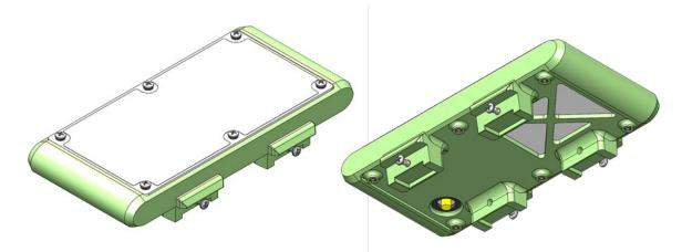
Figure 3-15. Example MP-compliant 4-pt Antenna Adaptor Assembly
