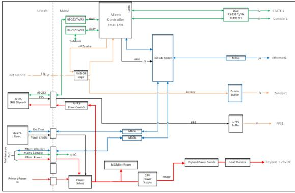
Figure E-4. MAIM Block Diagram for Stalker
