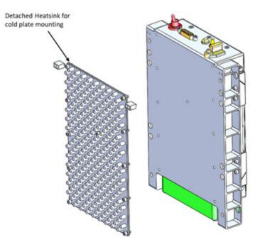
Figure 3-12. Heatsink Detached from the Bottom Surface of a Payload
