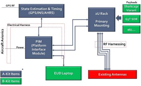
Figure C-1 C130 MPx System Architecture
