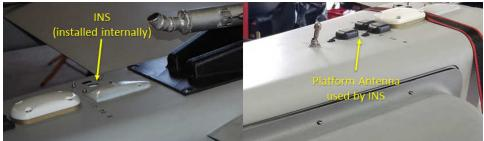
Figure D-11. Jump-20 INS Location and GPS Antenna
