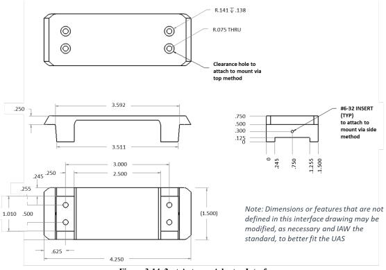
Figure 3-14. 2-pt Antenna Adaptor Interface
