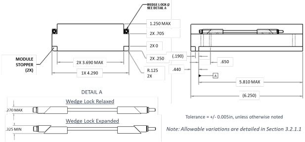
Figure 3-2. Detailed Dimensions of 1U Module
