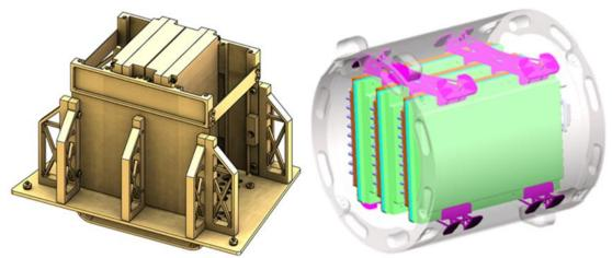
Figure 2-9. TigerShark 4U Primary Mount (left) and ScanEagle 3U Primary Mount (right)
