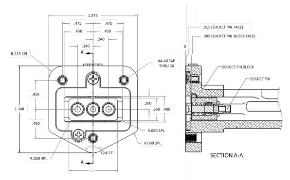
Figure 2-19. MP Array Antenna Mechanical Interface
