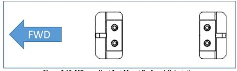
Figure 2-15. MP-compliant 2-pt Mount Preferred Orientation
