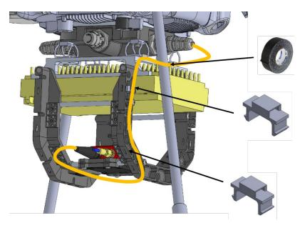
Figure F-20. SkyRaider MAIM-AHRS Cable Routing
