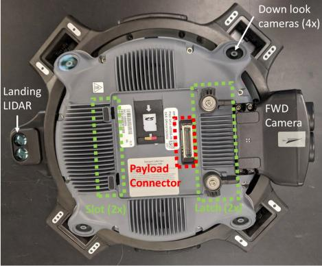
Figure F-18. SkyRaider Slot and Latch System
