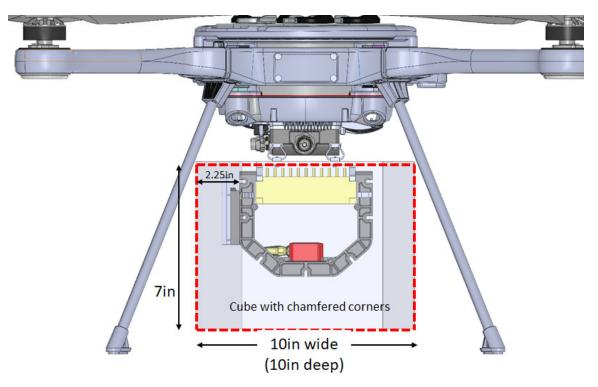
Figure F-15. Antenna Mounting Frame Allowable 2-pt Antenna Volume
