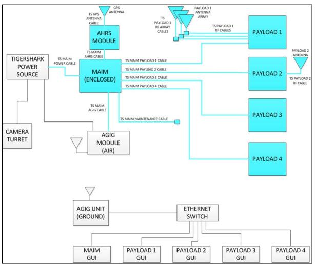
Figure C-2. System Diagram for MP-TigerShark
