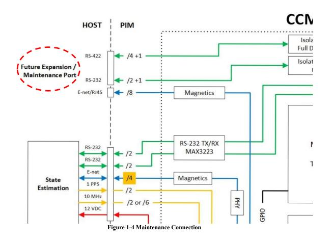
The maintenance connection shall have 1x RS-422, 1x RS-232, and one Ethernet connection
