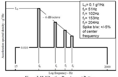
Figure 3-18. Vibration Requirement Pattern
