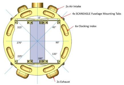
Figure B-8. ScanEagle Primary Mount Orientation
