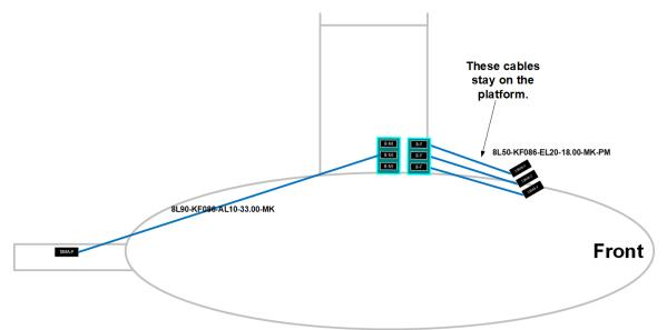
Figure E-22. Stalker RF Cables – Single Antenna Configuration
