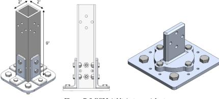
Figure B-9 CCM A-kit Antenna Adapters
