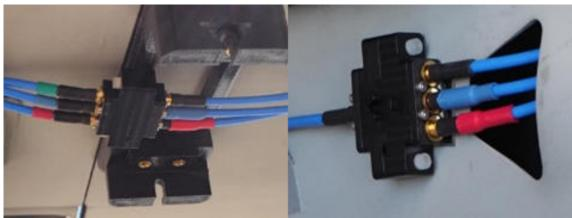
Figure E-25. RF Connector Block – 3-signal (left), 1-signal (right)
