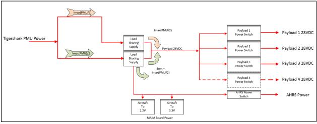
Figure C-5. MAIM Power Circuitry Block Diagram
