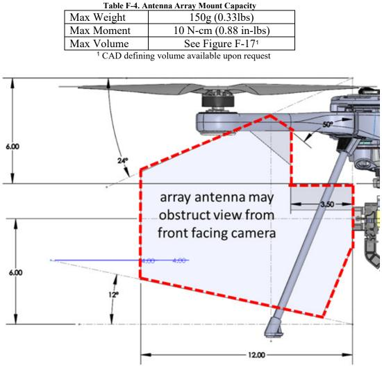
Figure F-17. SkyRaider Allowable Antenna Array Volume
