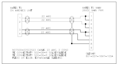
Figure D-18. MAIM Primary Power Cable Pinout
