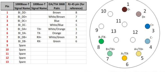
Chassis Connector (BOTH sides)D38999/20WB35PNCable Connector (BOTH ends)D38999/26WB35SN
