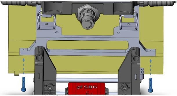
Figure F-8. SkyRaider Primary Mount - Payload Installation
