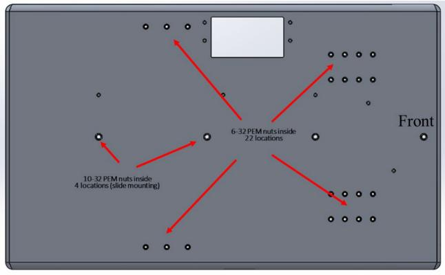
Figure 2-4 1U MPx Left Face (from the front face)
