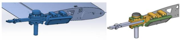
Figure C-12. TigerShark Wingtip Antenna Mount
