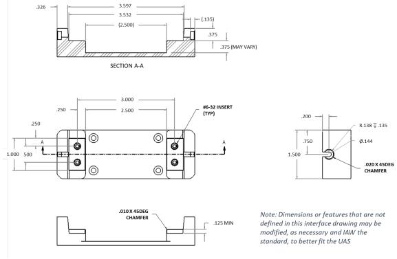
Figure 2-14. MP-compliant 2-pt Antenna Mount Interface
