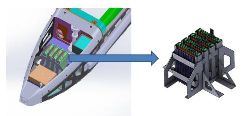
Figure C-9. TigerShark Primary Mount Installation
