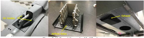
Figure D-10. Forced Convection Modifications
