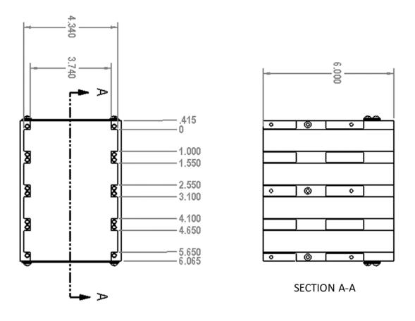
Figure 2-10. MP-compliant Rack Primary Mount Interface
