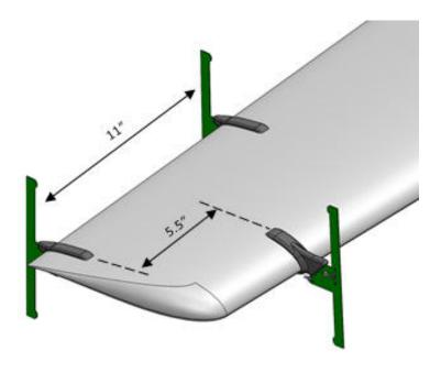
Figure E-27. Non-compliant SURFR3B Antenna Array Spacing
