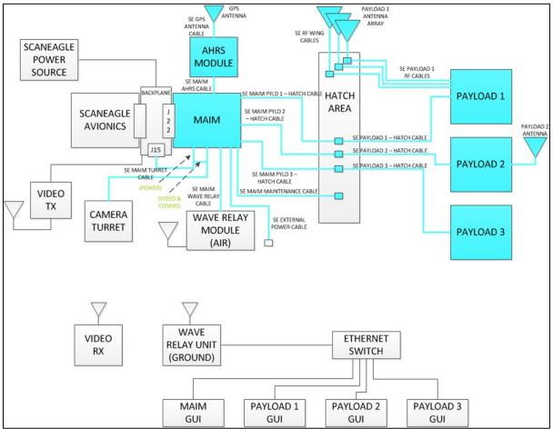
Figure B-2. System Diagram for MP-ScanEagle
