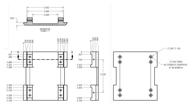
Figure 3-16. 4-pt Antenna Adaptor Interface
