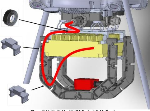
Figure F-19. SkyRaider MAIM-Payload Cable Routing
