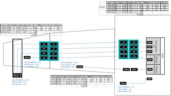
Figure D-23. Jump-20 Left RF Cables
