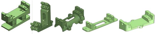
Figure 2-13. Example MP-compliant 2-pt Mounts
