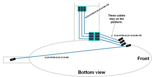
Figure E-24. Stalker RF Cables – Array Plus Configuration
