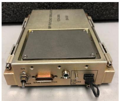
Figure 3-9. Example Payload Module Configured for Rack Mounting
