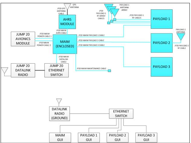
Figure D-2. System Diagram for MP-Jump-20
