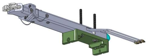
Figure B-12. Wingtip Antenna Mount
