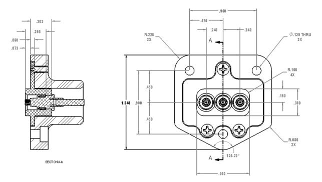
Figure 3-17. Array Adaptor Interface
