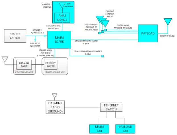
Figure E-2. System Diagram for MP-Stalker
