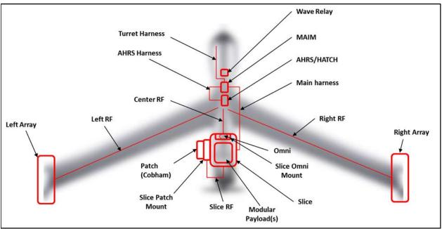
Figure B-1. Architectural Layout for MP-ScanEagle
