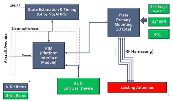
Figure D-1 CV-22 MPx System Architecture Concept
