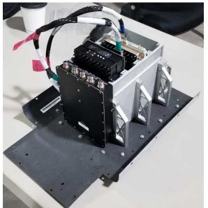
Figure D-7. Jump-20 Primary Mount with MAIM and Two Payloads
