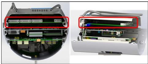
Figure B-6. MAIM Installed in ScanEagle
