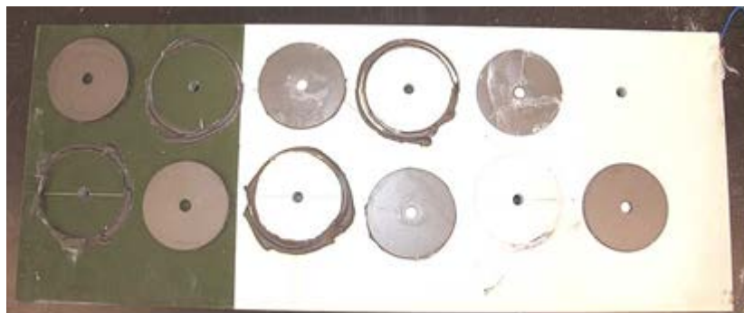
Figure 1b: Ti6Al4V washers placed against 2519-T87 aluminum protected by MIL-DTL-53022 (high solids, non-chromate) primer and MIL-DTL-81706 Type II conversion coating, after 2000 hours in ASTM B 117 neutral salt fog. Left side of panel has MIL-DTL-64159 topcoat (383 green).
