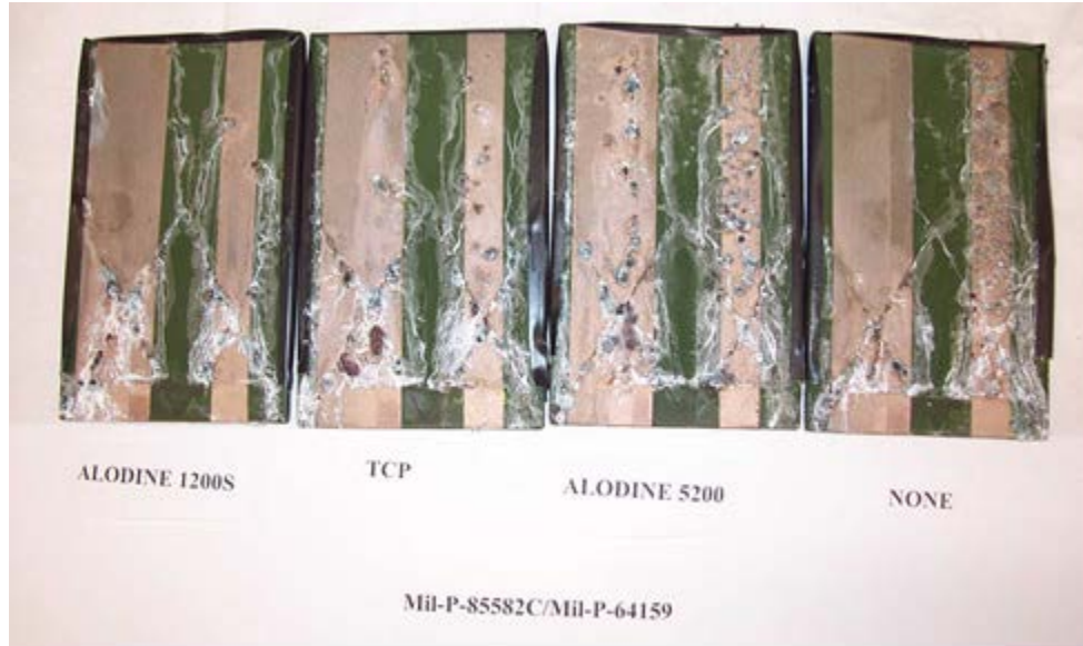
Figure 3b: Corrosion performance of MIL-PRF-85582 Class N primer and MIL-DTL-64159 topcoat in combination with silver epoxy paint on 2519-T87 aluminum with various pretreatments, after 7 days in ASTM B 117 neutral salt fog.
