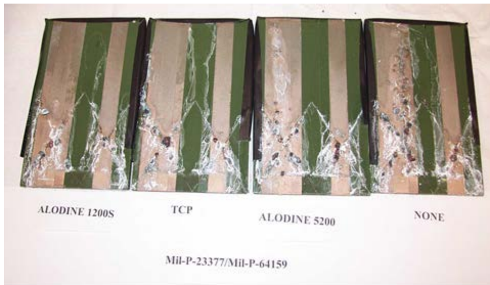
Figure 3a: Corrosion performance of MIL-PRF-23377 Class C primer and MIL-DTL-64159 topcoat in combination with silver epoxy paint on 2519-T87 aluminum with various pretreatments, after 7 days in ASTM B 117 neutral salt fog.
