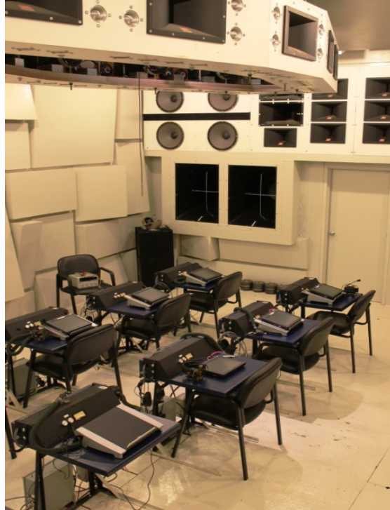
Figure 4. AFRL's VOCRES facility used to measure speech intelligibility performance
