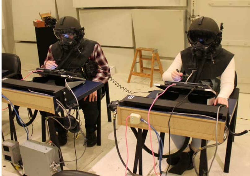
Figure 7. Subjects communicating via CCU for a high-noise, hardwired speech intelligibility measurement
