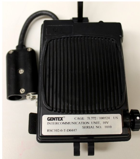
Figure 6. ICU (V)5 (10 volts) used for low-noise speech intelligibility measurements
