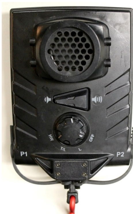
Figure 8. CCU used for high-noise speech intelligibility measurements
