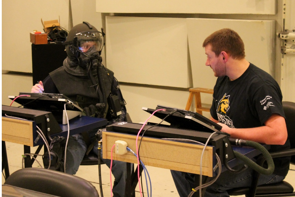
Figure 5. Subjects sitting one meter apart during a low-noise, over-the-air speech intelligibility measurement
