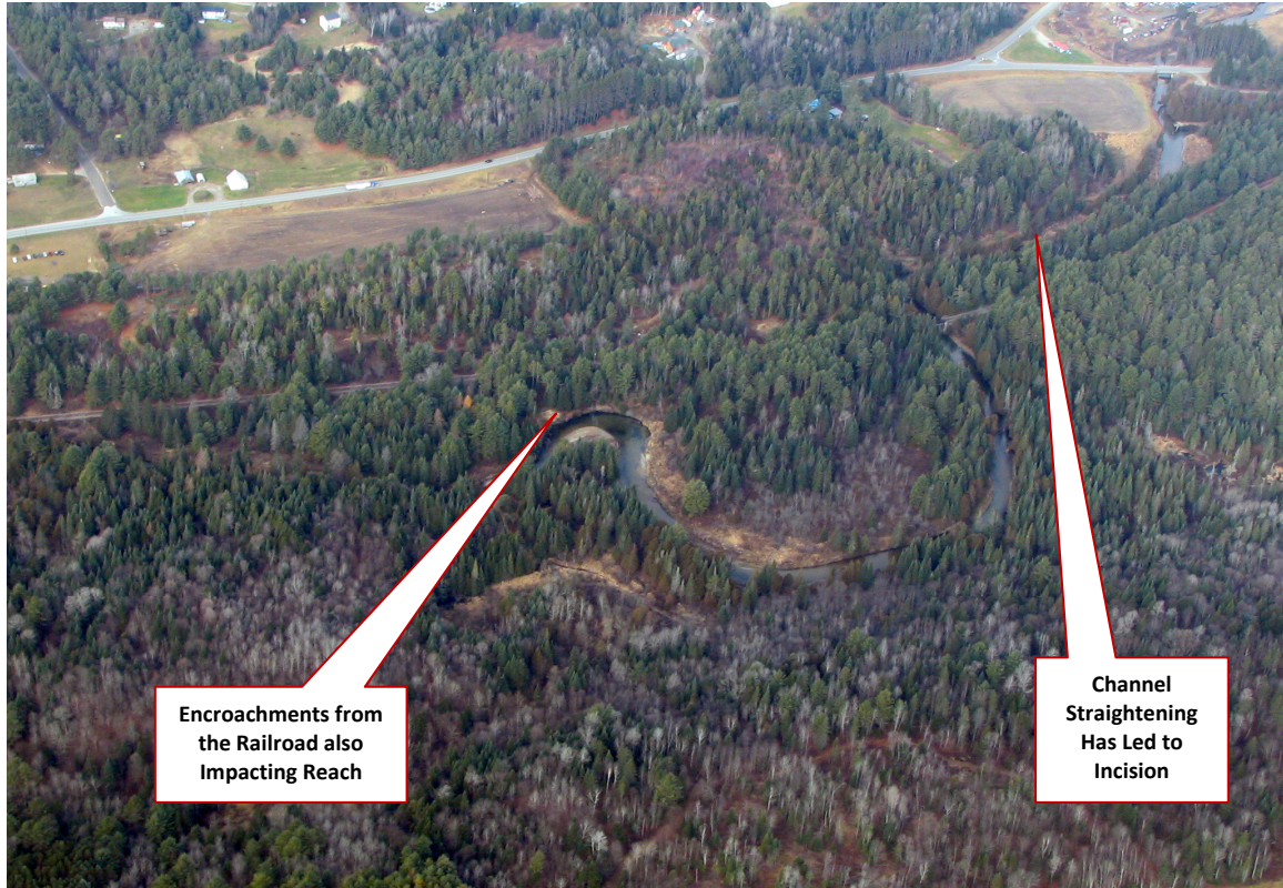
Figure 4.15 Reach T3.03 has corridor encroachments and channel straightening, which has led to channel incision
