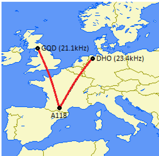
Figure 1. VLF signal propagation paths (DHO-A118 and GQD-A118) used in the study. Map adopted from the A118 channel; details at https://sidstation.loudet.org/channels-details-en.xhtml (last access: 18 May 2022).
