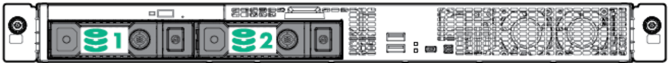
1-2 2 x LFF SATA/SAS/SSD Hot Pluggable and Non hot Pluggable Hard Drives Bays
