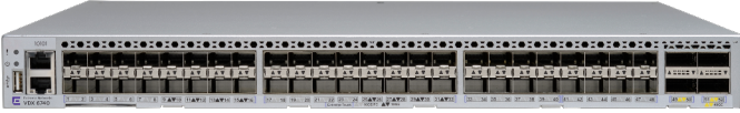
Figure 1: The VDX 6740 Switch provides 48 10 GbE SFP+ ports and four 40 GbE QSFP+ ports.
