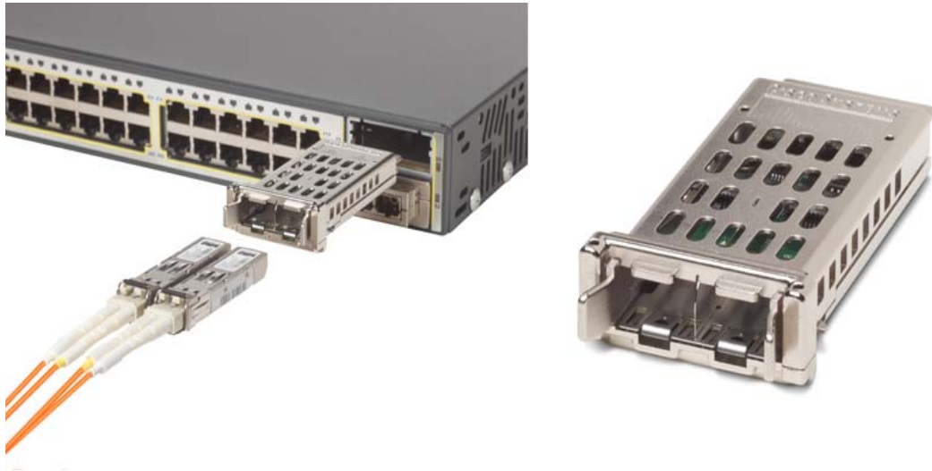
Figure 3. Cisco TwinGig Adapter Converting 10 Gigabit Ethernet X2 Interface into Two Gigabit Ethernet SFP Interfaces
