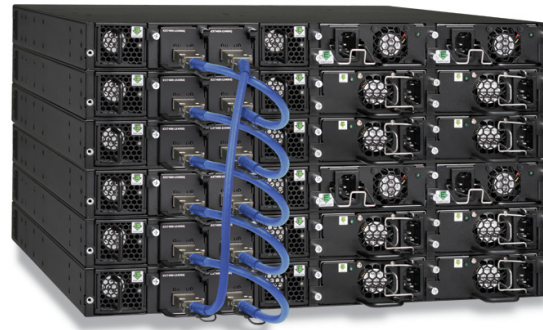
Figure 1: Up to 12 Brocade ICX 7450 switches can be stacked together using two full-duplex QSFP+ 40 Gbps ports that provide a fully redundant backplane with 960 Gbps of stacking bandwidth.
