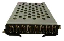
This auto-sensing tri-speed (10/100/1000 Mbps) module incorporates a space-saving design with mini-RJ21 connectors. It supports wire-speed performance of IPv4 and advanced MPLS features, and enables
