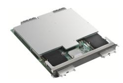
The 2-port 100 GbE module provides unmatched performance and scalability up to 32 wire-speed 100 GbE ports in a single Brocade MLXe-32 router and 16 wire-speed 100 GbE ports in a single Brocade MLX-32 router. This full-slot module complies with the IEEE 802.3ba standard and supports CFP-based short-reach and long-reach optics. Each 2×100 GbE module delivers 400 Gbps of throughput per module without compromising the performance of features such as IPv4, IPv6, and MPLS.
