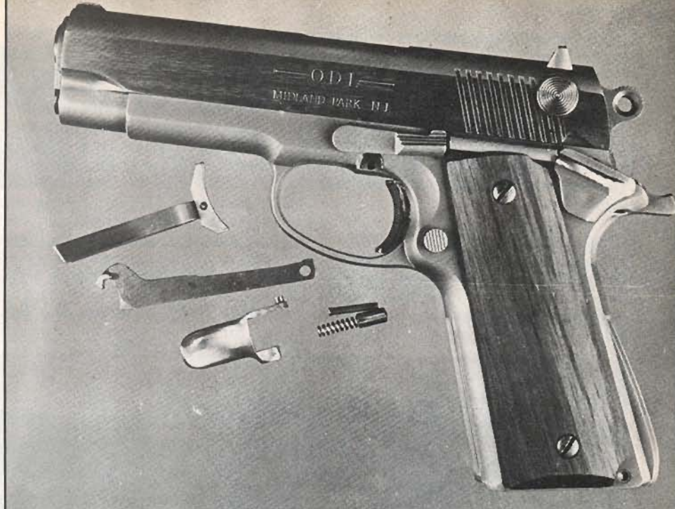
These are the parts that were taken out of the Viking II auto to turn it into a single-action pistol. Note the simplicity of the Seecamp conversion unit.
