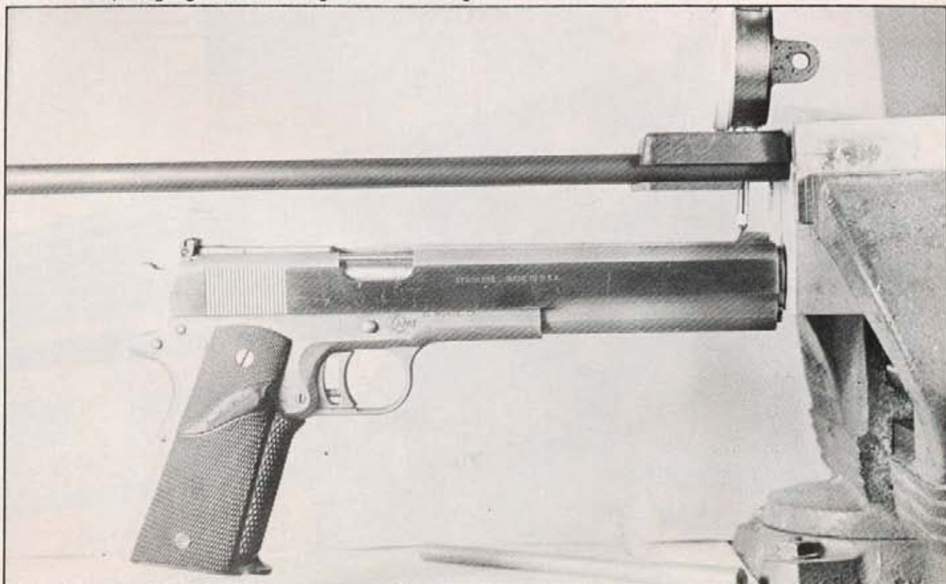
Millett Handgun Boresighter has a .45 Hardballer longslide on its barrel rod; the gauge measures height of the front sight.
