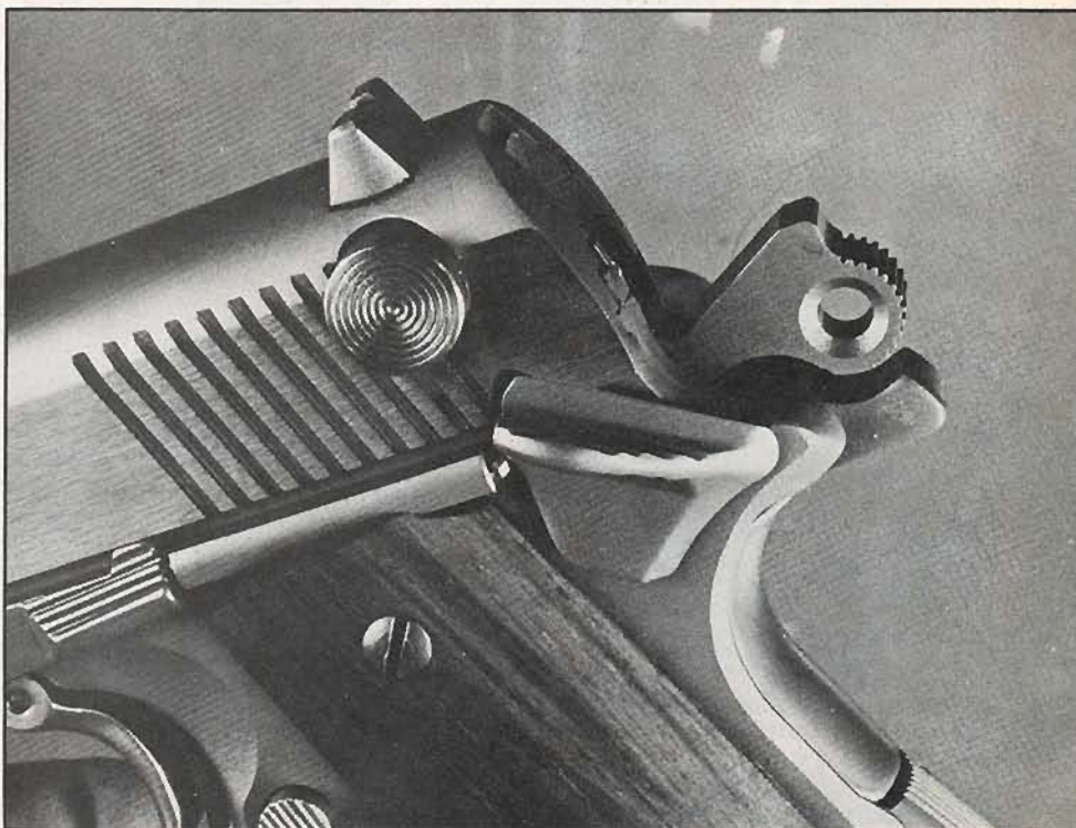
The firing pin safety has been moved to the left in the ON position. With the thumb safety UP and the hammer at full cock, the Viking II is extremely safe.
