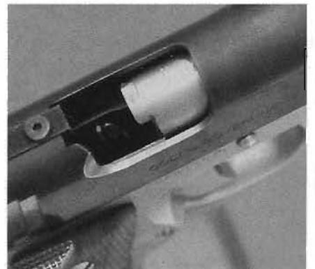
Cut in barrel locks into sight extension when barrel returns to battery.
