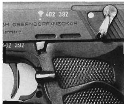
The "backward" safety on H&K's P9S is feature that takes getting used to.
