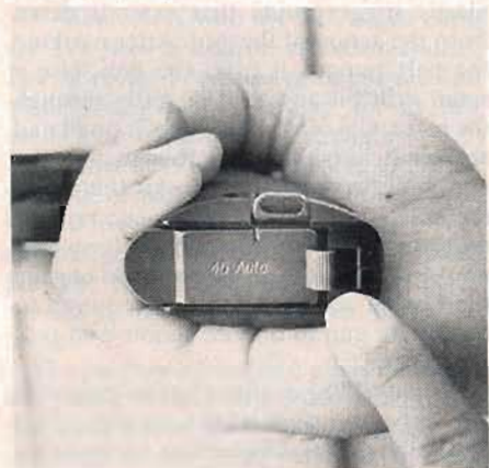
Butt release on BDA is same on P9S. Practice will make this release fast.
