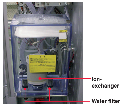
The Laser front (With front door opened)
