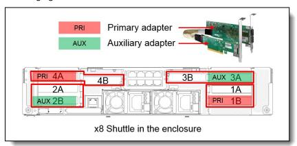
Figure 12. SharedIO adapters installed in the x8 shuttle
