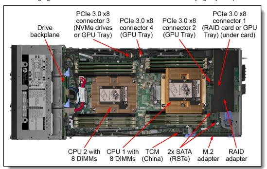
Figure 6. Internal view of the SD530 compute node
