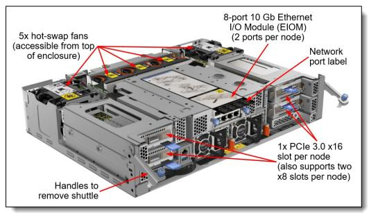
Figure 4. I/O Shuttle in the ThinkSystem D2 Enclosure
