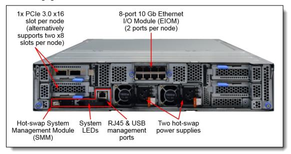
Figure 3. Rear view of the ThinkSystem D2 Enclosure
