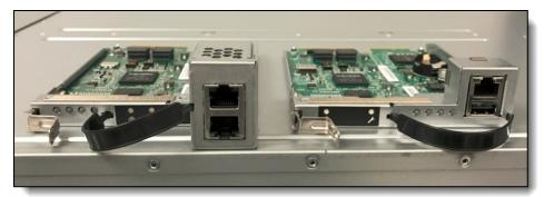
Figure 18. Dual-port SMM and standard (single-port) SMM
