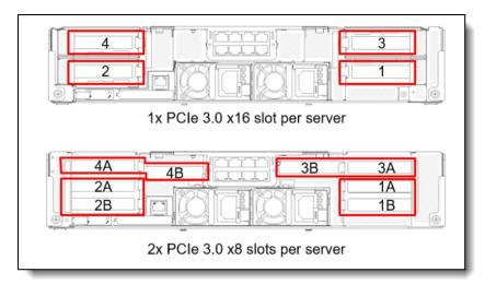
Figure 10. Location of the PCle slots at the rear of the Enclosure
