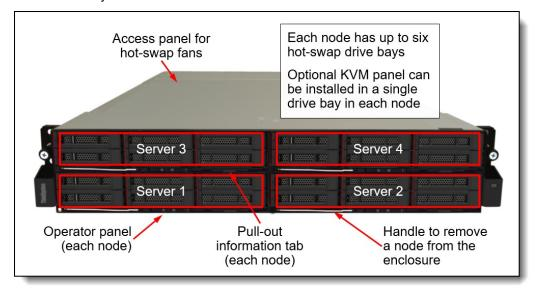
Figure 2. Front view of the ThinkSystem D2 Enclosure
