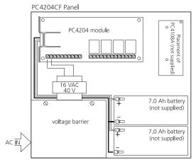
INSTALL BATTERY AND AC WIRING AS SHOWN ABOVE IMPORTANT: A minimum of 1/4" (7mm) separation must be maintained at all points between battery/primary AC wiring and all other wiring and connections.
