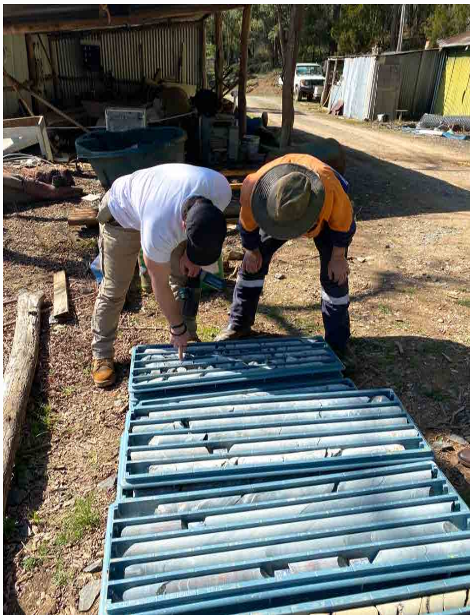
Stewart Govett and Chief Geologist Denis Walsh inspecting some of the 223 metres of DDH core from two drill holes showing massive sulphides that may contain gold and a large quartz vein intersected with pyrites and arseno-pyrites.
