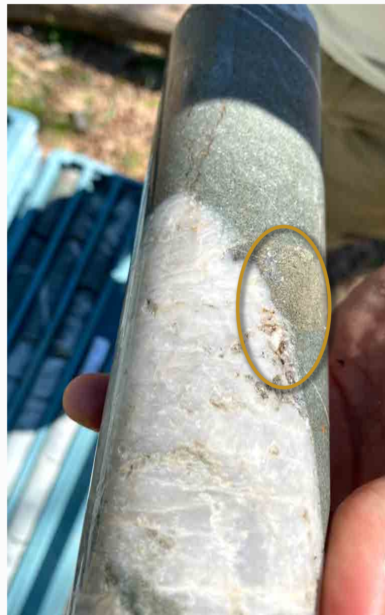
Stewart Govett and Chief Geologist Denis Walsh inspecting some of the 223 metres of DDH core from two drill holes showing massive sulphides that may contain gold and a large quartz vein intersected with pyrites and arseno-pyrites.
