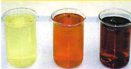
Orange juice microfiltered and then concentrated to 42° Brix and 62° Brix.
