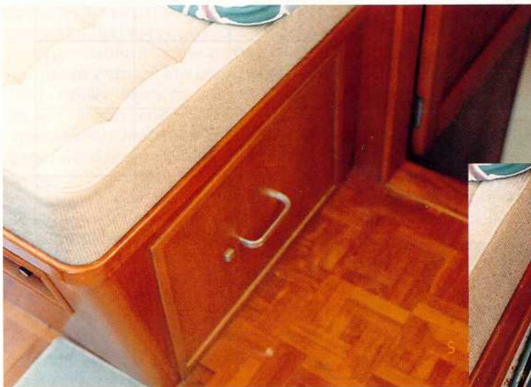
A standard legal file drawer was adapted and installed in lieu of the self-contained airconditioning unit which was moved to accommodate the new drawer size.
