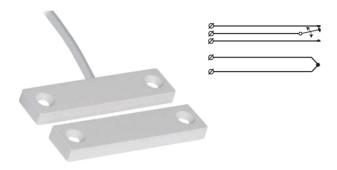
MC 746 is a small and thin magnetic contact with change-over (NC/NO) function that can be used in both alarm and access control systems for monitoring e.g. doors and windows against unauthorized opening.
