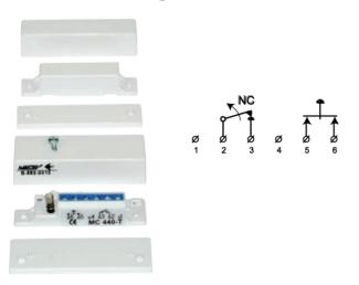
MC 440-T is a surface mount magnetic contact with NC function and with 6 screw connections. It can be used in both in alarm and access control systems for monitoring e.g. doors and windows against unauthorised opening.
