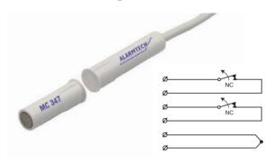
MC 347 is a universal magnetic contact with double NC function that can be used in both alarm and access control systems for monitoring e.g. doors and windows against unauthorized opening.
