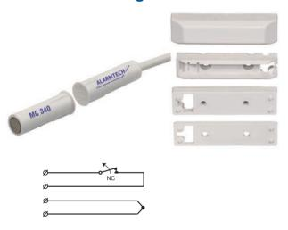
MC 340-S3 is a universal magnetic contact set with NC function that can be used in alarm and access control systems for monitoring e.g. doors and windows against unauthorized opening. Both the contact and the magnet part are in a water proof (IP 67) plastic housing.
