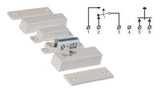
MC 446 is a surface mount magnetic contact with change-over NC/NO function and with 6 screw connections. It can be used in both in alarm and access control systems for monitoring e.g. doors and windows against unauthorised opening.
