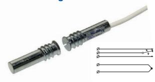
MC 246 is a universal magnetic contact with change-over (NC/NO) function that can be used in both alarm and access control systems for monitoring e.g. doors and windows against unauthorized opening.
