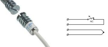
MC 255-LSZH is a universal magnetic contact in small format with NC function and halogen-free cable that can be used both in alarm and access control systems for monitoring e.g. doors and windows against unauthorized opening. Both the contact and the magnet part are made of Al-alloy and formed in the shape of a threaded screw, which allows for easy installation into wood or plastic. The magnetic contact has a rotating screw system which protects the cable from mechanical stress in tight spaces.
