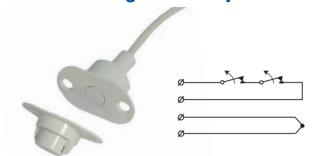
MC 370-S12 is a high security magnetic contact set with NC function that can be used in both alarm and access control systems for monitoring doors and windows against unauthorized opening.
