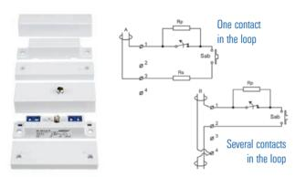
The magnetic contact MC 440 with 2 built-in resistors for a balanced circuit. When installing the magnetic contact it is easy to select if one resistor or both should be used (see wiring diagram) For quick and easy installation the magnetic contact comes with screw terminals with wire protection. It is equipped with tamper protection against unauthorized opening.
