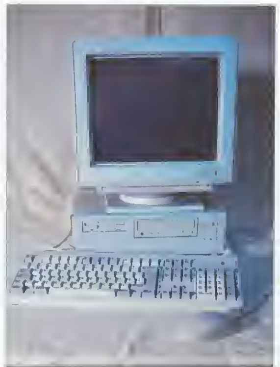
The A7000 boasts a compact and robust design. The ATAPI CD-ROM drive shown here is optional – the A7000 can take a single expansion card, but only if it has no CD-ROM drive, as they occupy the same physical space inside the machine.
