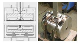
Fig 2: HCX focusing doublet design and fabrication.
