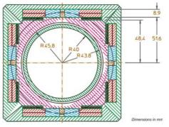
Fig. 3: Racetrack design for IBX (dimensions in mm).
