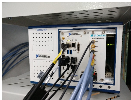
Figure 1: Data acquisition board and PXIe chassis for BTB position on-line measurement.
