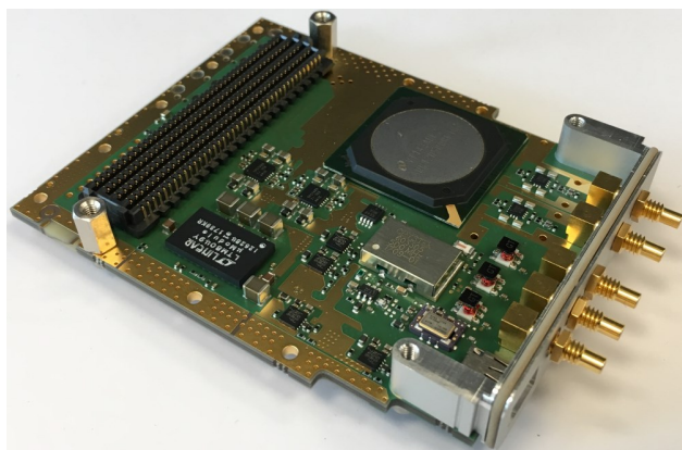
Figure 1: New DFMC-DS500 digitizer board.
