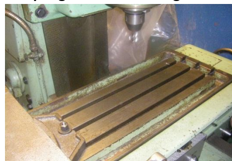
Fig. 7.12 - Clamping table from a milling machine
