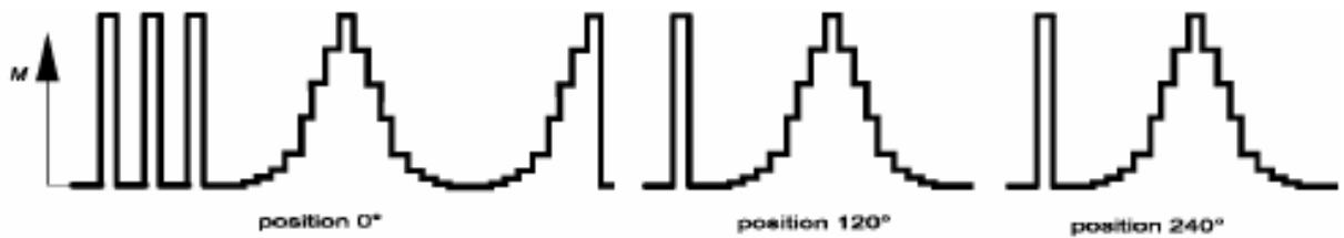
Fig. D.1: Example of preloadings and sequences for torque measuring devices with a minimum 8 steps and U < 0,1\%
