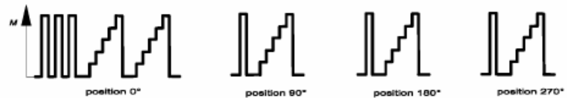
Fig. D.3: Example of preloadings and sequences for torque measuring devices with square drive, a minimum 5 steps, only increasing series and 0,1\% = U < 1\%
