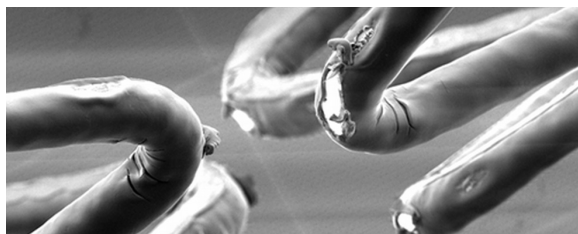
Cracks and bare metal areas on DES
