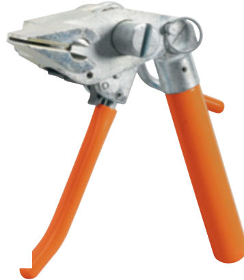
WTC075 Designed to install ¼" to ¾" wide Free-End Clamps. The lightweight, ratchet-action tool tension cuts and secures the buckle tab.
