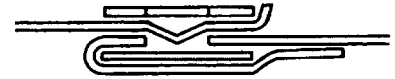
The tail is formed into a fold lock behind the buckle. The tool forces a dimple in the band into a hole in the buckle.
