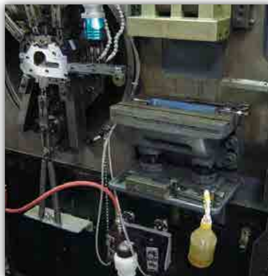
Minimum quantity lubrication used on a tapping workcenter
