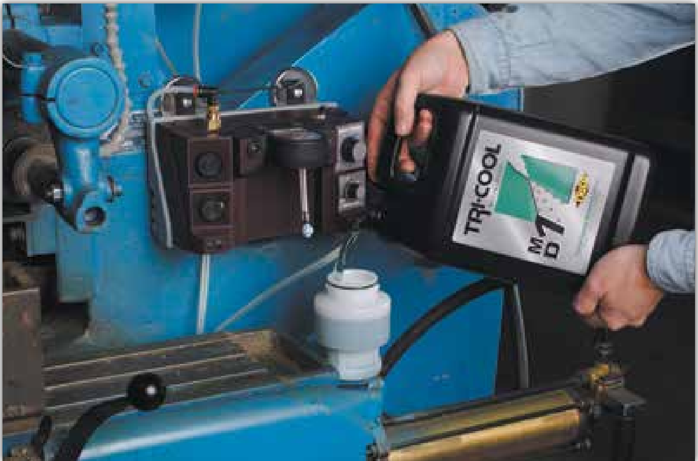
Micro-dispenser being filled with Tri-Cool MD-1 lubricant
