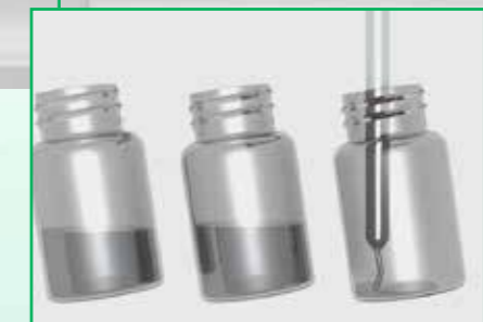
Tilted reagent vial positions to reduce reagent wastage
