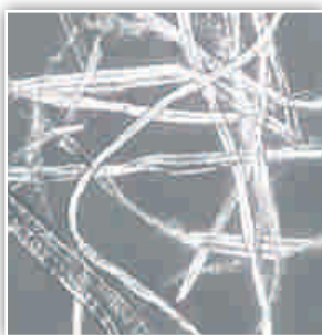
Loose Cellulosic Fibres under a Microscope
