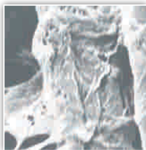
Cellulosic Fibres Bound in a Filter Paper under a Microscope
