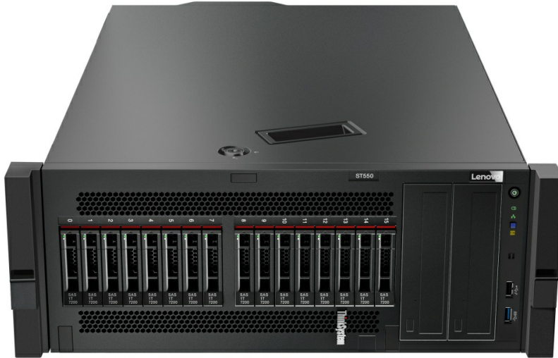
Figure 20. ThinkSystem ST550 with Rack Conversion Kit installed
