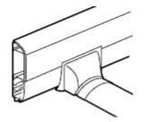
For branching from skirting-trunking 140x35 mm to floor duct Cat. No. 032800
