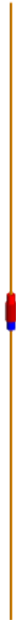
Figure 1: A 3D view of the dipole with a voltage source in CADFEKO.
