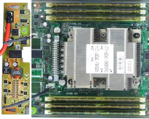
48V Converter Board
