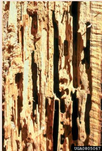
Slika 27. Rovni sistemi velike črne gozdne mravlje ( Camponotus herculeanus ) (foto.: R. Werner, USDA Forest Service, www.forestryimages.org) Figure 27. Galleries of carpenter ant ( Camponotus herculeanus )
