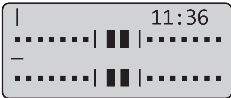
Fig 3.3 Display when level appears thus "coarse mode"
