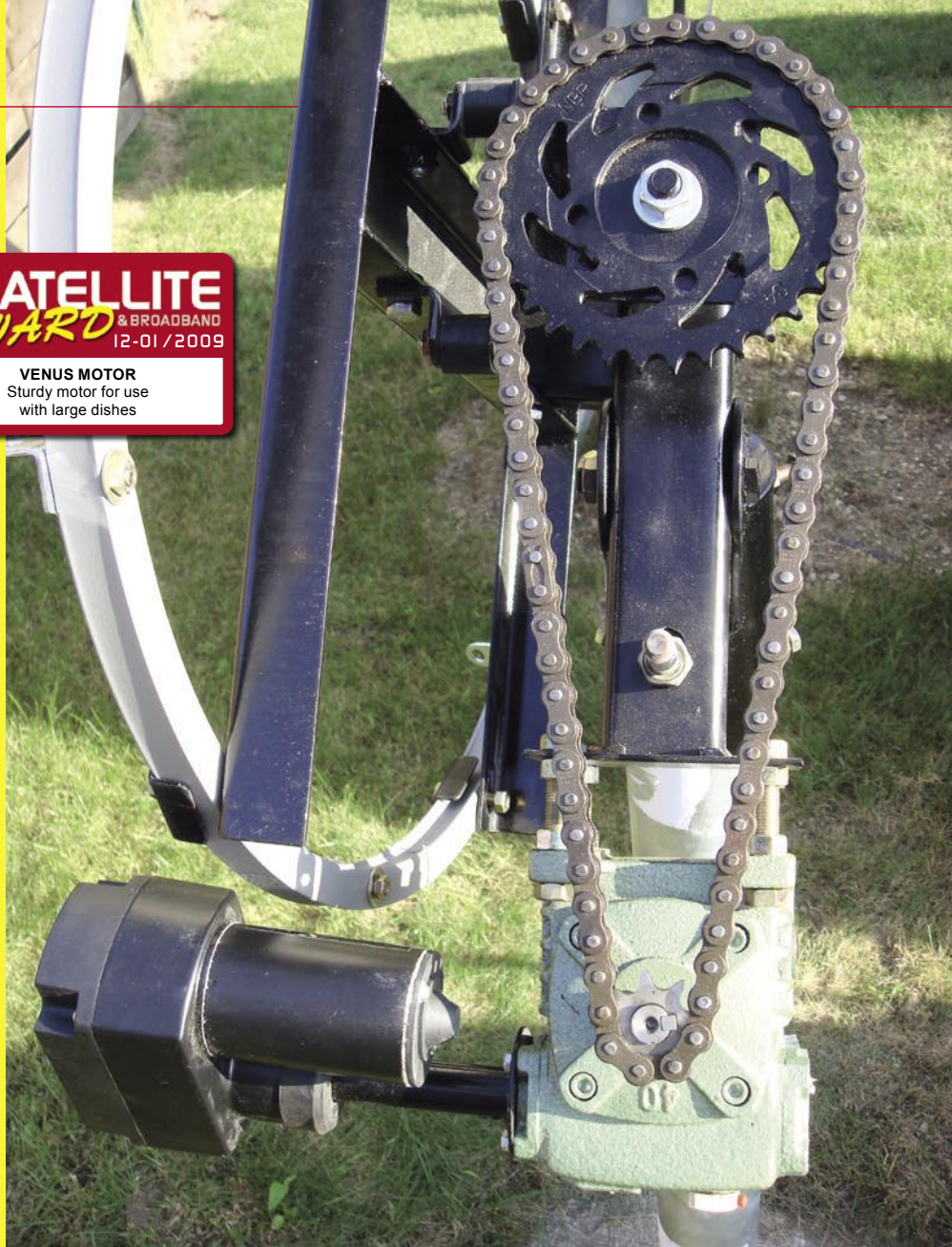
■ Motor from PT. Subur Semesta with chain transmission from the gearbox to the axis
