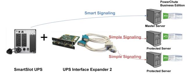
**Note**: For the sake of this FAQ, 'Protected Server' refers to additional secondary servers that are shutdown serially by the UPS Interface Expander 2.
