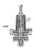
**Type 64SR** - Is a high pressure regulator which has an integral relief valve. As such it may be used as a final stage regulator on high pressure systems. It may also be used as a first stage regulator when set at 10 psig or less.
