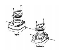
**Gaskets & Screws for Float Gauges**
