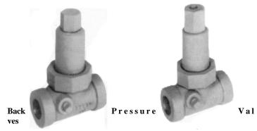
Thes e valves are soft seated, holding a differential back pressure on liquid meters. Type N120 is installed after the meter, and it holds a back pressure on the meter until vapor is forced back to the tank through the vapor eliminator. In this way vapor cannot form within the meter during liquid delivery.
