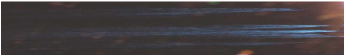
Fig. 3 Snapshot multiple filamentation in glass K8 when exposed PFC at a distance of 90 m from the end of FMF.
