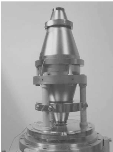
Fig. 6 Photograph of one of the silicon resonators resting on a stiff tripod support (a). Individual frequency instability determined from a three-cornered hat comparison of the two silicon based laser systems (Silicon 2 and 3) working at 1.5 \mu\text{m} [8] and a 698 nm laser stabilized on a 48 cm long ULE resonator [9].
