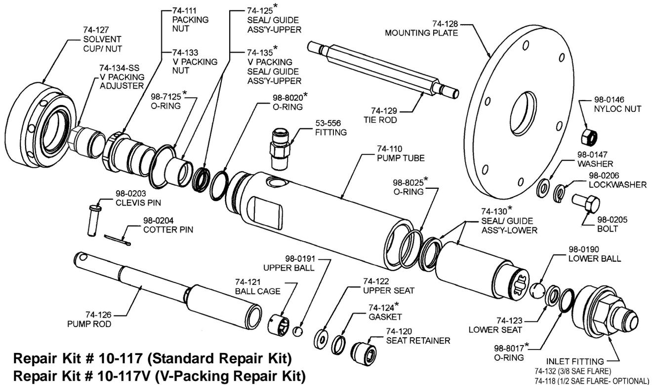
**Repair Kit # 10-117 (Standard Repair Kit)**
