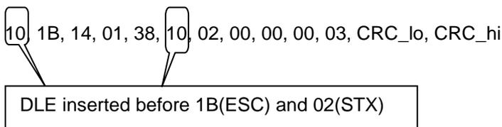
DLE inserted before 1B(ESC) and 02(STX)
