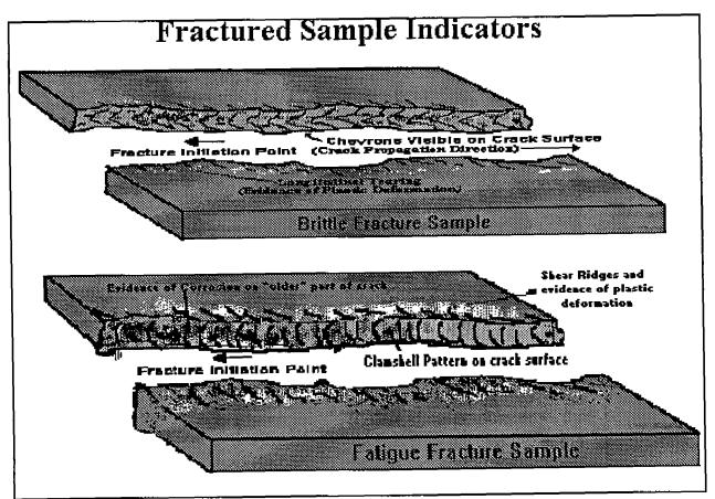
Figure 16 Fracture Mode Identification Sketch
