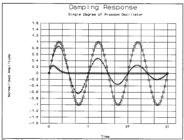
Figure 10 Response of SDOF Oscillator With Various Degrees of Damping
