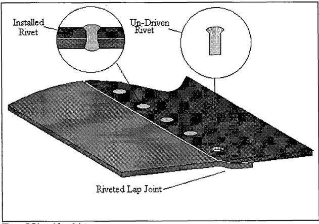
Figure 7 Riveted Lap Joint
