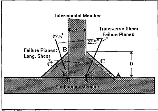
Figure 3 Fillet weld failure planes
