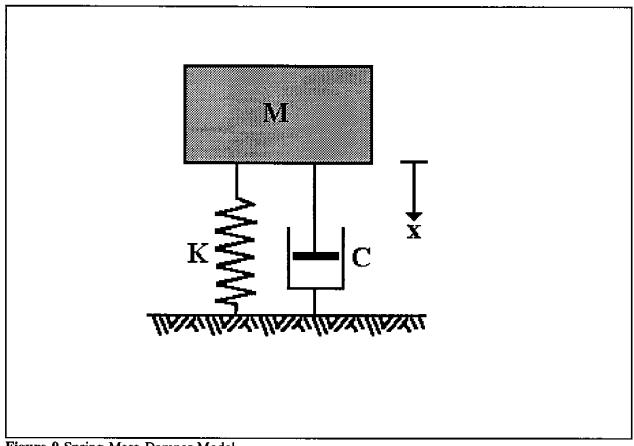
Figure 9 Spring-Mass-Damper Model
