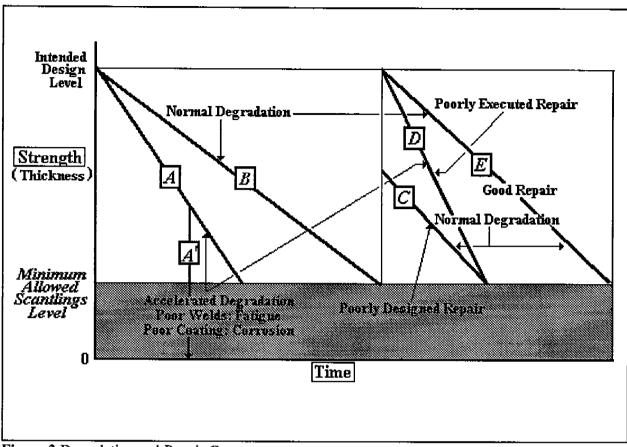
Figure 2 Degradation and Repair Curves
