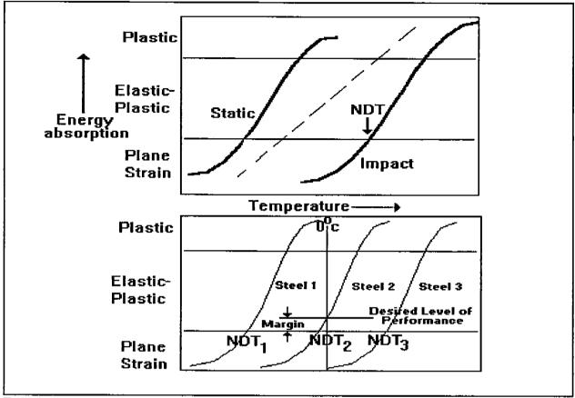
Figure 18 Brittle Fracture Transition Curves
