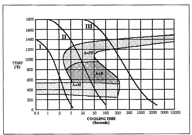
Figure 6 Steel Crystalline Transformation/ Cooldown Curves
