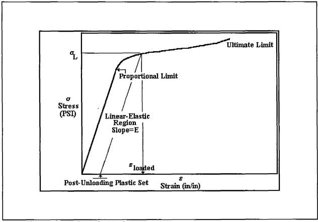
Figure 13 Stress-Strain Curve for Metal
