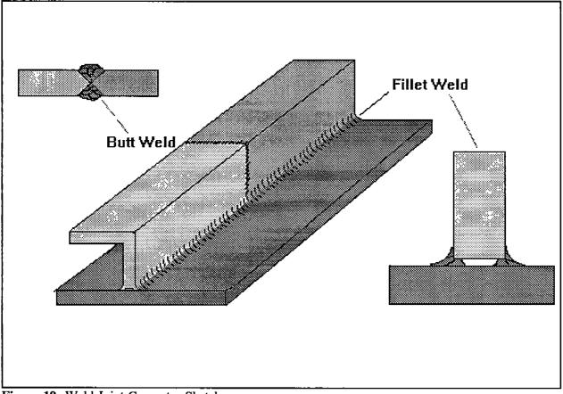
Figure 19 Weld Joint Geometry Sketch
