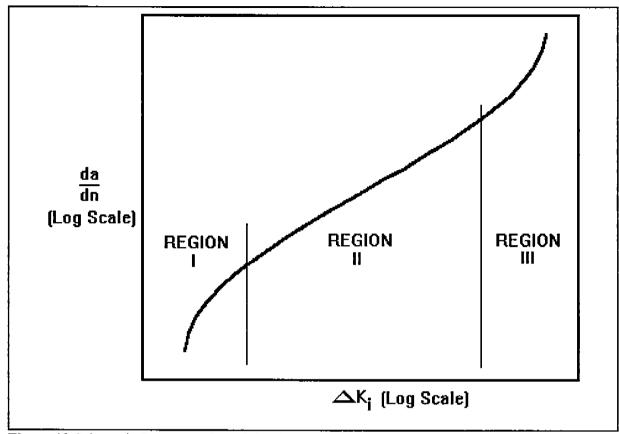
Figure 12 Schematic Representation of Crack Growth in Steels
