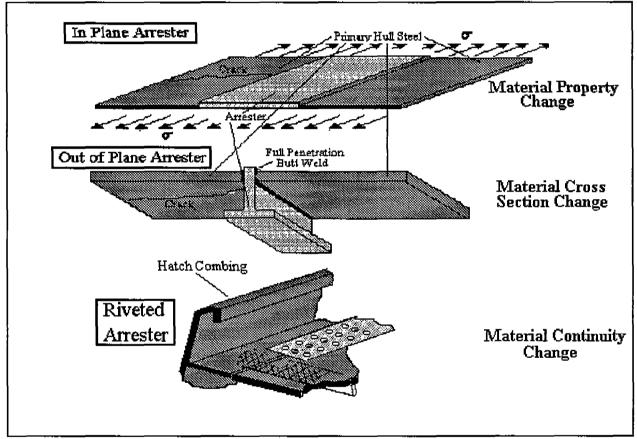
Figure 14 Crack Arrest Schemes
