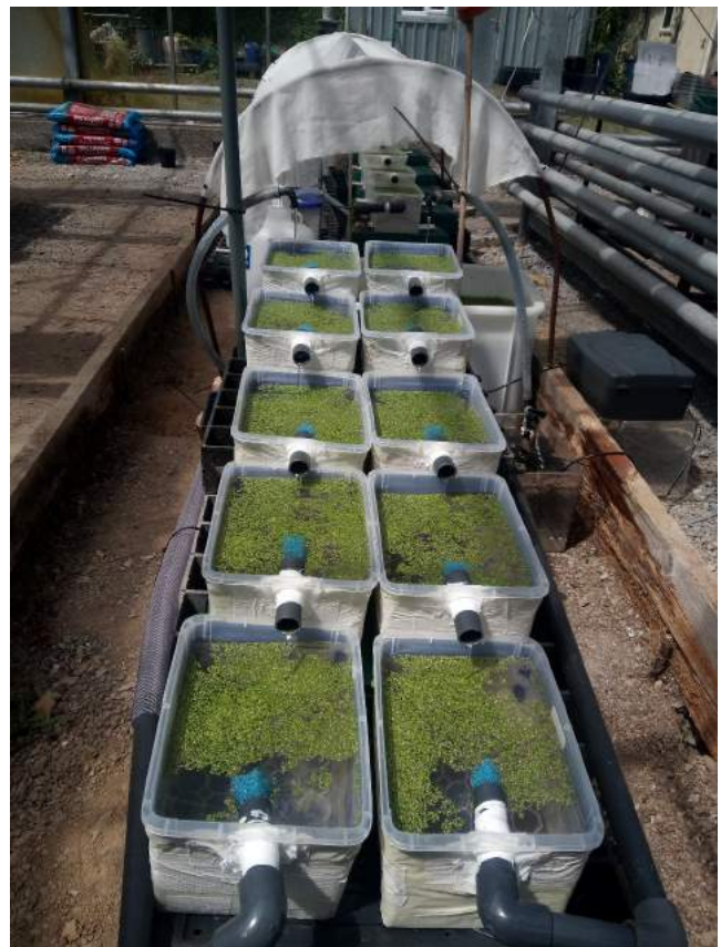
Figure 4. A simple cascading system at UCC, used for small scale experiments.
