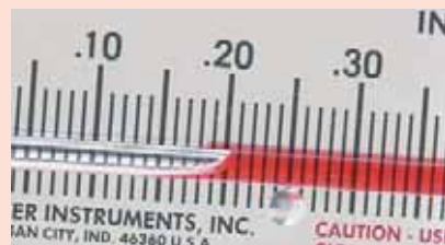
Fig. 2-5. Portion of the scale of a Dwyer No. 250.5 solid plastic inclined manometer shown full size. Parallax free reading is made by aligning meniscus with its reflection in the polished scale.
