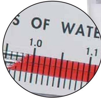
Fig. 8-1. No. 424-10 Inclined-Vertical Manometer, 0-10" water range. The inset shows a segment of the inclined scale in actual size. No. 424-5, 0-5" water range is similar.
