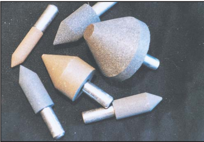
MOUNTED POINTS FOR THE EX-CELL-O CENTER LAPPING MACHINE (60 DEG INCLUDED ANGLES) 1/2" X 1-1/4 SHANKS
