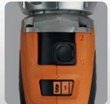
Predetermined torques can be set via changing the gear and setting the power setting step
