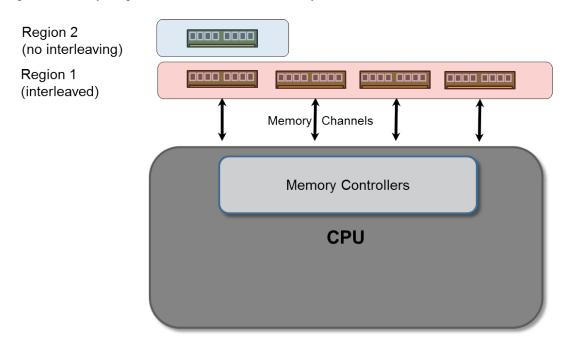
Figure 13. A memory configuration that is unbalanced across memory channels
