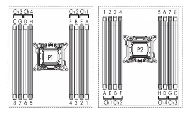
Figure 6 shows the memory slot configuration for the 12 slot 2P ProLiant Gen8 servers that use the E5-2400 series processors. These servers have only three memory channels per processor. The first memory slots for each channel on each processor are the white memory slots (A, B, and C). You should populate the memory for 12 slot servers using the same general rules as those for 24 and 16 slot servers.
