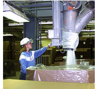
Small polypropylene pellets are packaged and shipped to manufacturing facilities that create plastic products.
