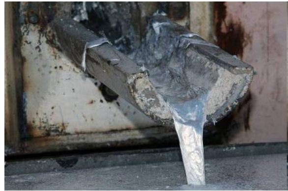
Scrap aluminum is melted to remove impurities.
